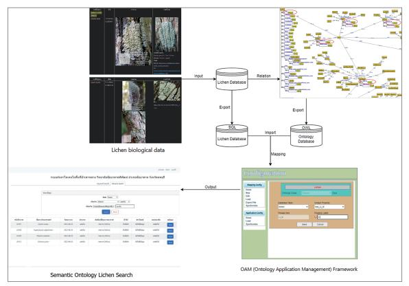
Figure 5 – The system architecture.
